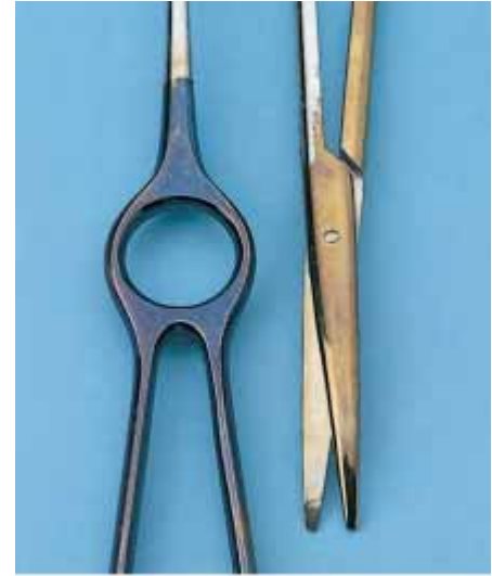
Anlauffarben - Bunt schillernde Silikatbeläge Rainbow colors - colorful shiny silicate coatings
